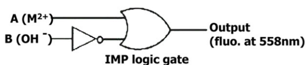
Fig. 4 Logic circuit for the two-input IMP gate.
